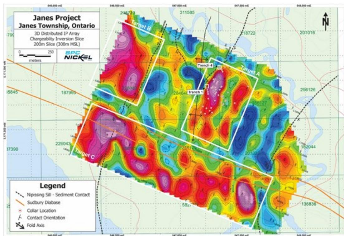
**Figure 1:** 3D Distributed IP Array Chargeability Inversion Slice (200 m) of the Janes Property with interpretations and target areas. Note: For the survey, an average sea level (Mean Sea Level - MSL) of 300 m was used.
