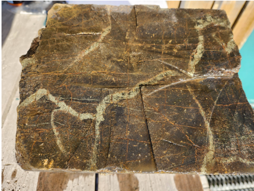
Fig. 1: Massive sulphide (pyrrhotite and chalcopyrite) sample from Pyrrhotite Lake area. Note that grab samples are selective by nature and may not be representative of mineralized zones. Source: SPC Nickel
