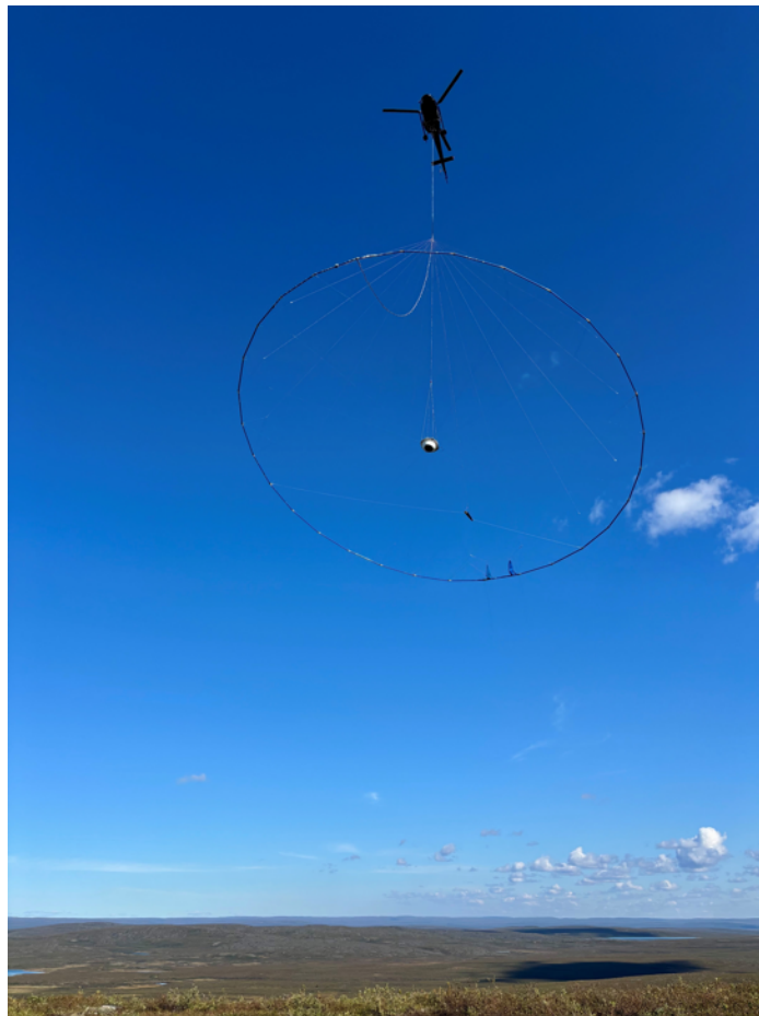
Fig. 4: HeliTEM airborne geophysical survey (Xcalibur Geophysics). Source: SPC Nickel
