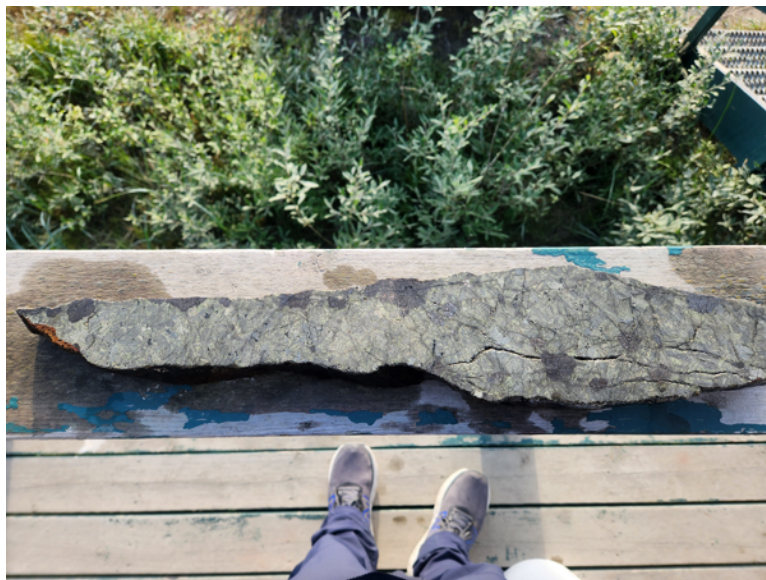
Fig. 2: Massive sulphide (chalcopyrite, cubanite, pyrrhotite, pentlandite) sample from the Spears Lake area. Note that grab samples are selective by nature and may not be representative of mineralized zones. Source: SPC Nickel
